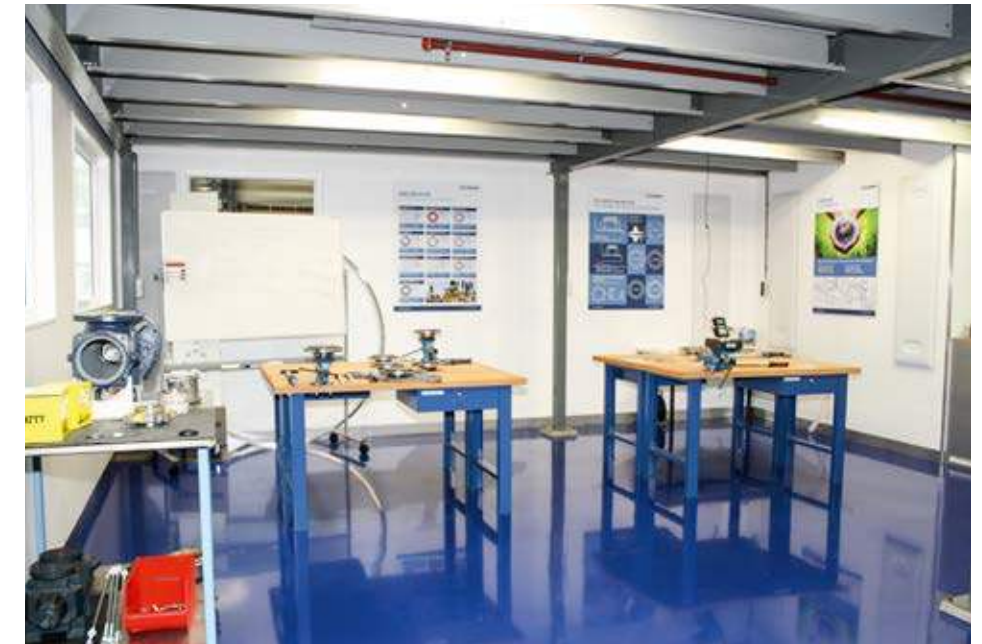
Worktables for flange management and assembly training include, amongst others, a torque wrench calibration station and practice flanges
