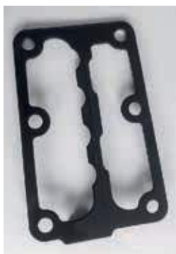
Gasket cut from rubber- coated steel
