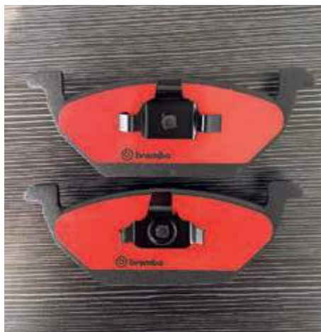
RCM employed as a shim on disk brake pads
