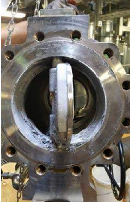
Due to their design, butterfly valves are especially prone to the effects of scaling
