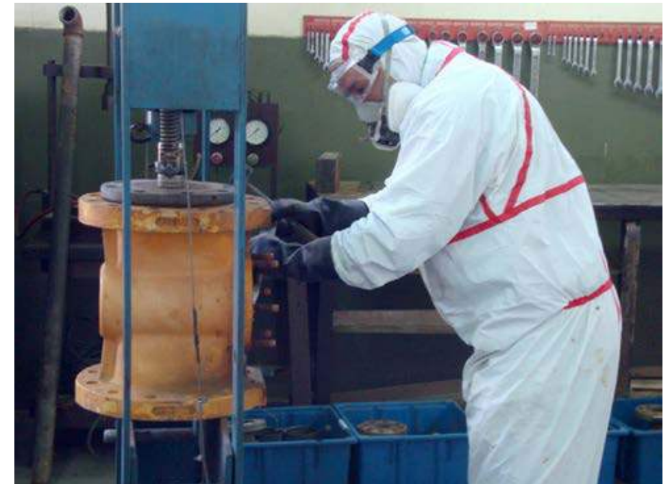
10:00 pm: KLINGER technical personnel disassembling an 8" sleeved plug valve
