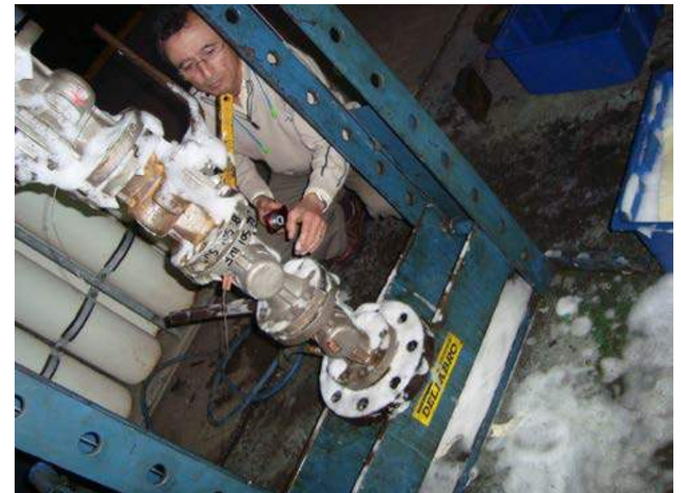
4:30 am: The valve inspector carries out the leakage test as per ANSI 598
