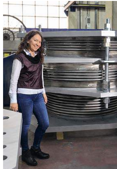
Bediha on site with an expansion joint.
